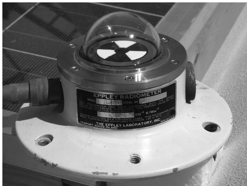
FIGURE 2.29 Photograph of a pyranometer.
